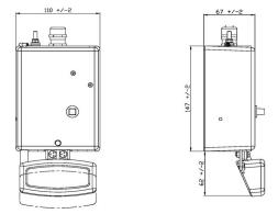
Brake handle swtich releases an emergency stop. Design more robust thanks to a strengthened guide allows operation even in situations of stress.
